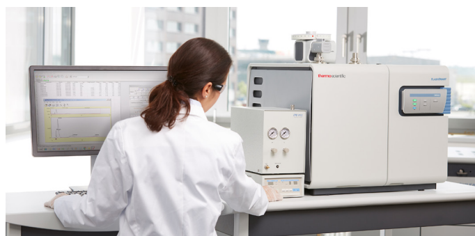
Figure 1. Thermo Scientific FlashSmart Elemental Analysis coupled with Flame Photometric Detector (FPD).
