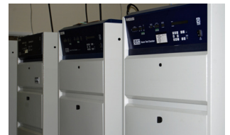
Q-SUN Xe-1 and Xe-3 test chambers in the lab.
