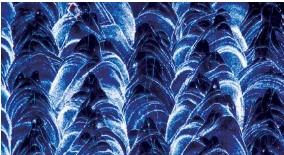
Additively manufactured titanium alloy (Ti-42Nb), viewed indarkfield illumination at 500x magnification ~ Dennis Pede; Institute for Materials and ApplicationTechnology (IWAT), Germany
