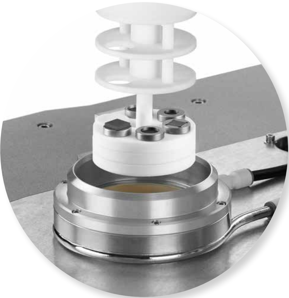
Patented Multi-sample Carousel with Flexible Tray and Adaptors
